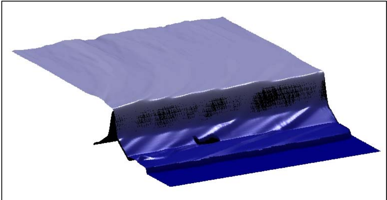
Figure 15-41. Side angle view of numerical waves overtopping the levee near the Paris Road Bridge. The levee is shown as the submerged black shape. View is looking towards the southwest; waves are from the east (left side of image)
