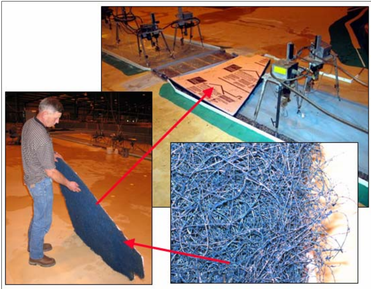
Figure 12-20. Debris field simulation using fiber mesh material
